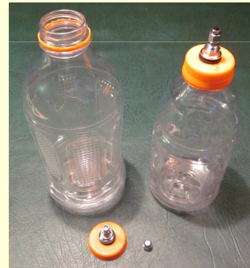
Gatorade bottles, Shrader tire valves, tire filler chock = portable pressure vessels
